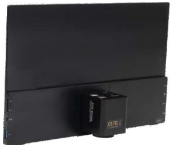
Back View of MTD1080P1330 Displayer and HDMI Camera's Connection
