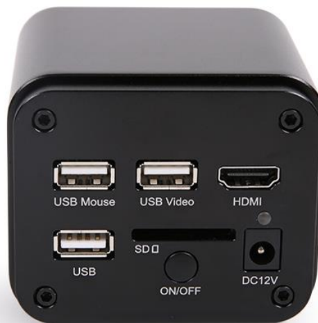
Figure 2 Available Ports on the Back Panel of the Camera Body
