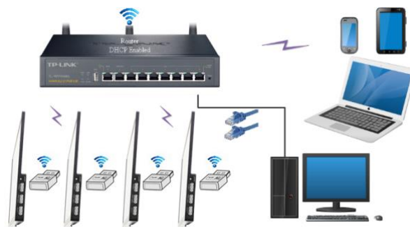
Figure 10 Multi ISVIS4K8MPCA Series All-in-One Cameras Connecting to the Router through the WiFi Style
