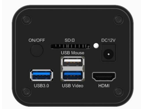
Figure 2 Available Ports on the Back Panel of the Camera Body
