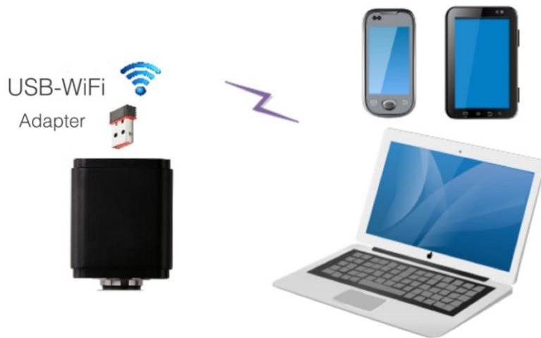
Figure 7 The PC or Mobile Device Connect to the Camera through WiFi
