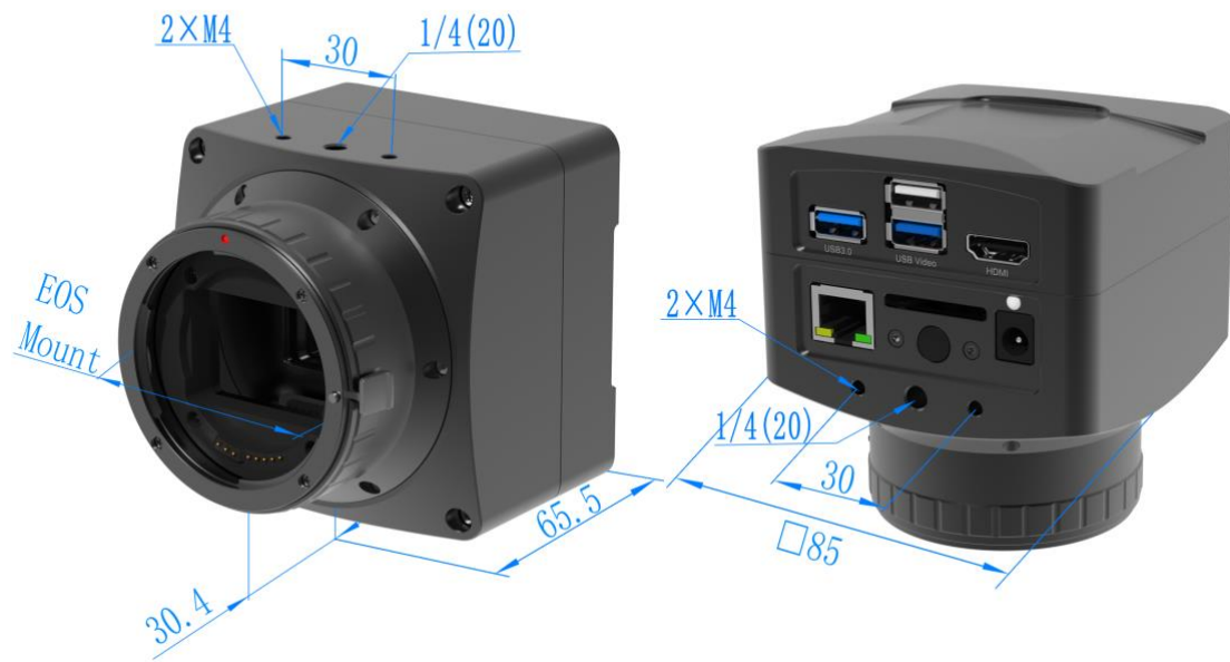
Figure 8 Dimension of UPROAF4KUHD16MPCA_EF
